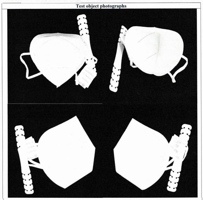
The samples delivered and tested were marked with the following information: KINGYI OP01 FFP2 NR EN149:2001+A1:2009 *mark* CE 2163.
